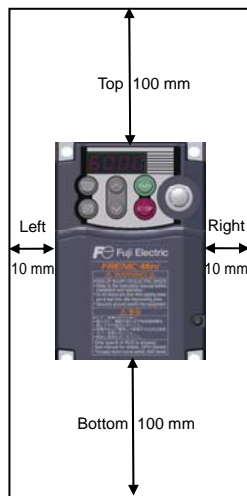
Figure 2.1 Mounting Direction and Required Clearances
